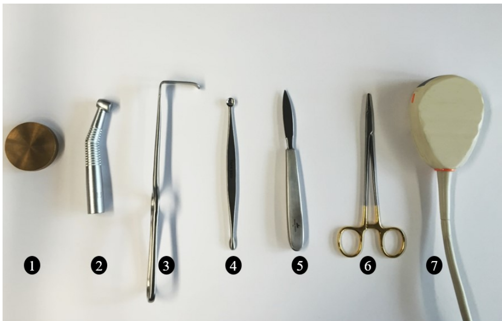
Figure 3.16: Sources of distortions: (1) a 5 \times 1\text{cm} brass disk, (2) a dental drill body, (3) a Langenbeck hook, (4) a bone curettes (5) a scalpel, (6) needle holder and (7) an ultrasound probe. In this measurement, the different sources of distortions were put between the sensor and field generator for both the commercial system and the experimental setup. A test phantom was utilized to fix the catheter location. The distance between the sensor coil and the distorter was fixed to 1\text{cm} .
